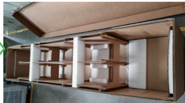
Linear Module Packaging After Improvement
